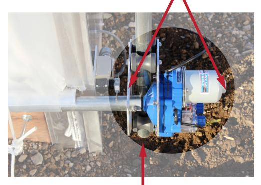
2-3" between the edge of the greenhouse and the guidewheel unless you are using roll lock. When using roll lock you need an external limit switch to control the downward movement of the motor.
